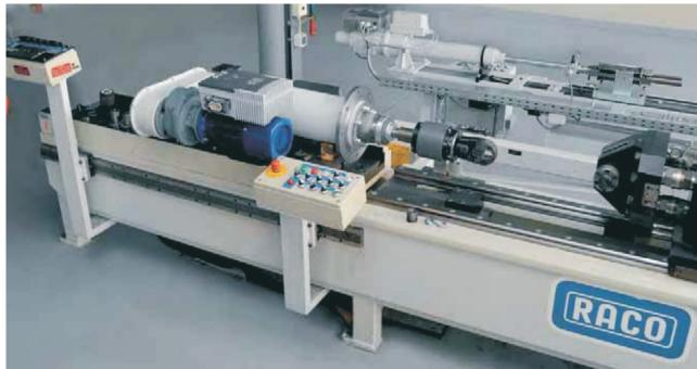
RACOmatic® offers continuous monitoring of the actuator system. Parameters such as temperature, voltage, and power consumption provide information about the condition of the actuator system. All safety features have been integrated into the RACOmatic® system. Tailored-to-suit maintenance work can be performed as needed; in critical situations the actuator can be stopped automatically.
